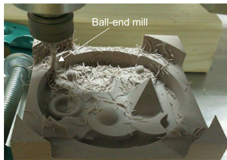
Fig. 11 Machining scene of machining robot RV1A using zigzag-based CLS data shown in Fig. 7 (left); resultant surface (right)
