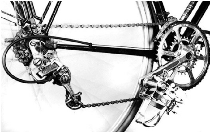
Fig. 4 Derailleur mechanism for changing sprockets sizes, Brown [33]
