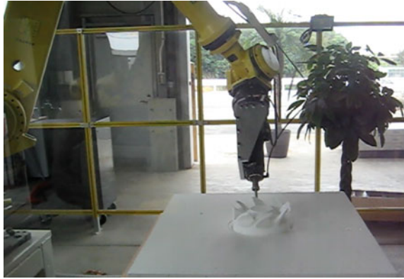
Fig. 2 Machining robot based on FANUC R2000iC
